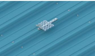
FROGLINK INSTALLED LESS THAN 2M FROM BOTH SIDES OF ROOF SHEET EDGES REQUIRE 4X12G ADDITIONAL SCREWS TO SECURE ROOF SHEETS INTO PURLINS ON BOTH SIDES THAT FALL UNDER 2M
