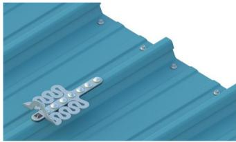
FROGLINK INSTALLED LESS THAN 2M FROM ROOF SHEET EDGES REQUIRE 4X12G ADDITIONAL SCREWS TO SECURE ROOF SHEETS INTO PURLIN ON SIDE THAT FALLS UNDER 2M
