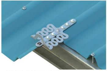
**OPTION 2: FROGLINK MOUNTED ONTO ROOF SHEET** AND PURLIN BY 6 RIVETS AND 1X14G SCREW THROUGH CENTER HOLE.
