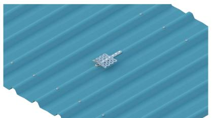
FROGLINK MUST BE INSTALLED ON ROOFS WITH MINIMUM OF TWO PURLINS/BATTENS WITH A PURLIN/SCREW LINE ABOVE AND BELOW THE ANCHOR POINT
